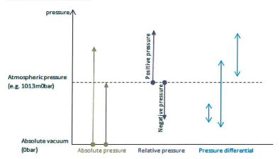
The absolute pressure is defined as the pressure which occurs with the absolute vacuum (0bar) as basis. At sealevel the absolute pressure is the same like the atmospheric pressure (1013mbar).
